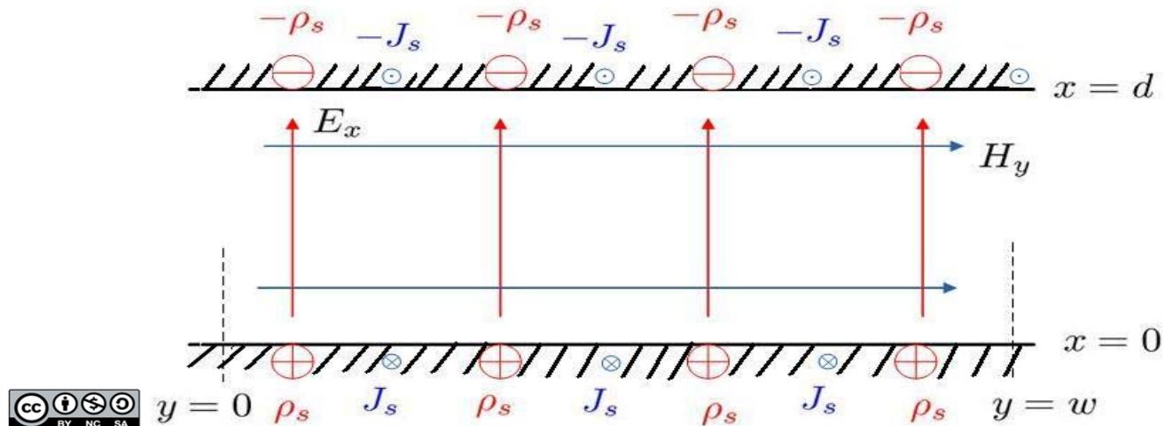
$$\int_0^d E_x(z, t) dx = E_x(z, t)d = V(z, t) \quad (1)$$
