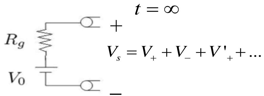
$$\begin{aligned} V(z=0, t=\infty) &= V_s = V_+ + V_- + V'_+ + V'_- + \dots \\ &= V_+ (1 + \Gamma_L) (1 + \Gamma_L \Gamma_s + \Gamma_L^2 \Gamma_s^2 + \dots) \\ &= V_+ (1 + \Gamma_L) \frac{1}{1 - \Gamma_L \Gamma_s} \end{aligned}$$
