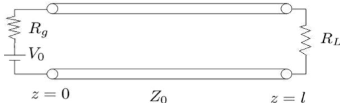
$$V(z,t) = V_+ \left( t - z / v_p \right) + V_- \left( t + z / v_p \right)$$
