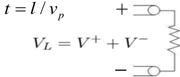
$$V_- = V_+ \boxed{\frac{R_L - Z_0}{R_L + Z_0} = \Gamma_v} V_+$$
