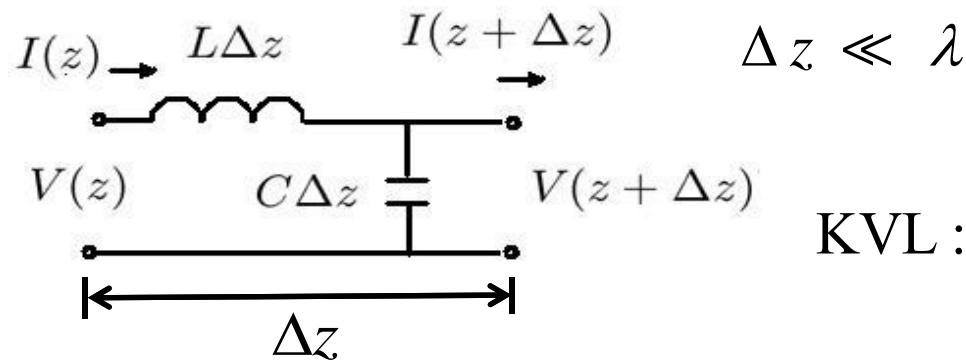
$$\text{KVL : } V(z) = L\Delta z \frac{\partial I(z,t)}{\partial t} + V(z + \Delta z, t) \stackrel{\cong}{=} V + \frac{\partial V}{\partial z} \Delta z$$
