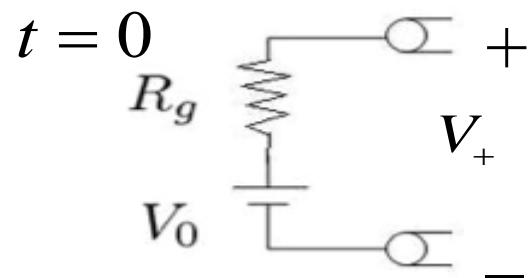
$$\Rightarrow V_+ = V_0 \frac{Z_0}{R_g + Z_0}$$
