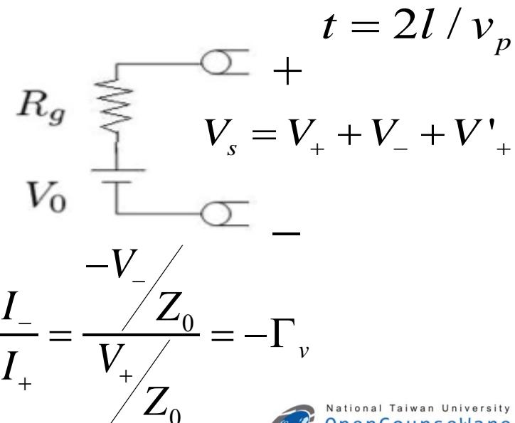
current reflection coefficient:  $\Gamma_I = \frac{I_-}{I_+} = \frac{-V_-}{V_+} / Z_0 = -\Gamma_v$
